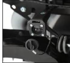
EU043 External magnetic charging receptacle
