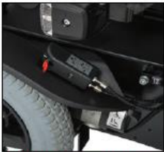
EF020 Caster wheel swivel lock
